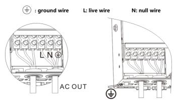
Note: use thick ground cable as far as possible (with cable section not less than 4mm²), place the ground point to be close to the all-in-one machine as far as possible and choose shorter ground wire to the greatest extent
