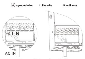
③ Correctly connect AC output wire in accordance with cable sequence and terminal position shown in the figure below. Please connect the ground wire at first, and then live wire and null wire. The ground wire is connected to the ground screw hold through Oshaped terminal.
